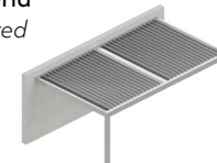
Lama paralela a pared Louvers parallel to the wall
