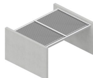
Lama perpendicular a pared Louvers perpendicular to the wall
